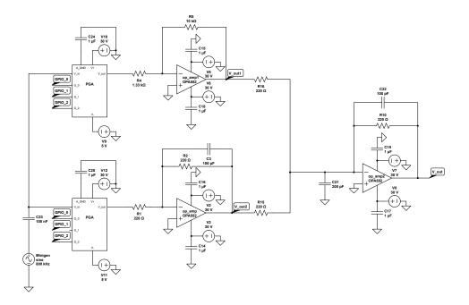
Figure 2: Amplifier circuit design to vary voltage within range  $1V_{pp}$  to  $60V_{pp}$ .
