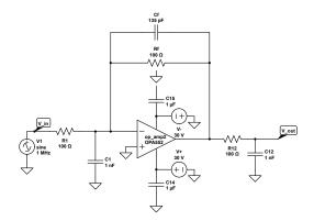
gain of 1 op-amp with frequency compensation and phase shift correction.
